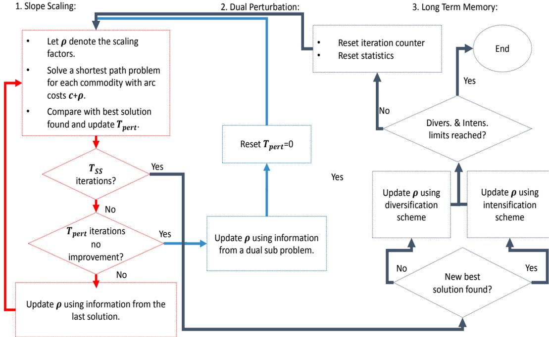
Figure 4: Slope scaling heuristic for MUFND
